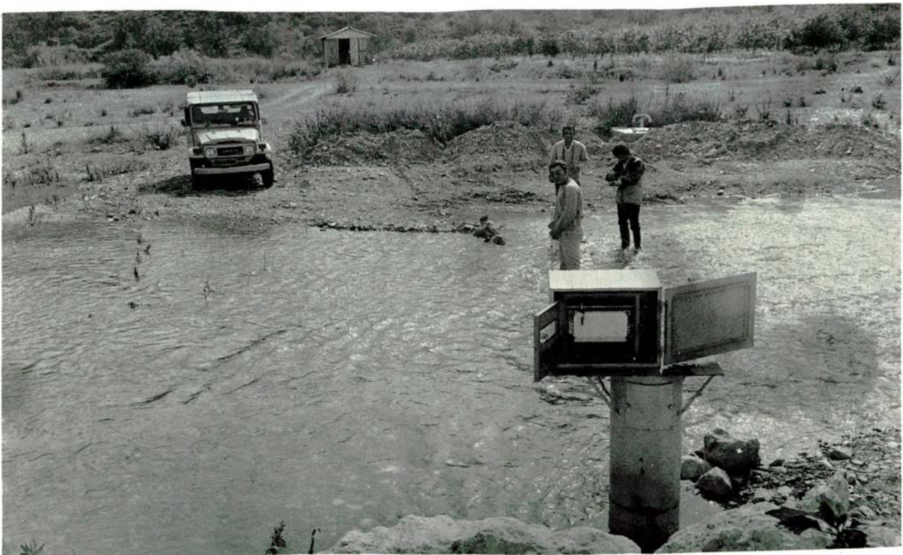
Measurement of flow in Yermasoyia river 2 km downstream the reservoir to determine infiltration rates. WDD Photo D46-7, 4.4.83.
