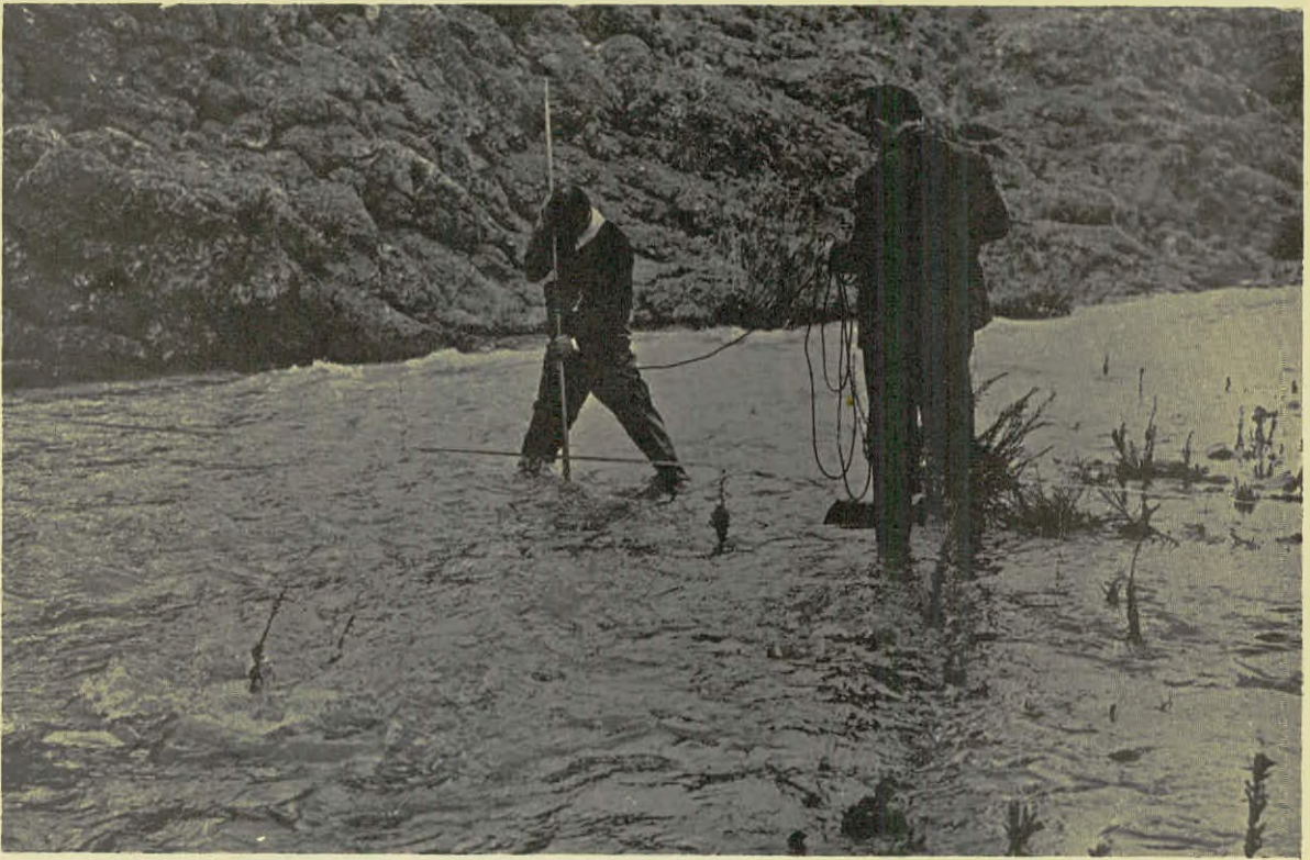
Current meter measurement of flood flow by wading in the Akaki river near Malounda
