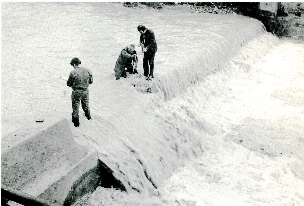
Measuring the flow of Akaki river with a Current Meter
